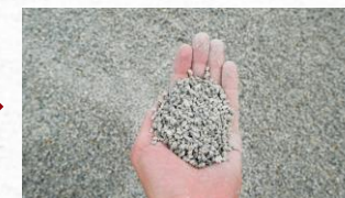
Maskin Sand 0/2F - 0/2 – 0/4 – 0/8 Grov Tilslag 2/4 – 4/8 – 8/16 – 16/22
