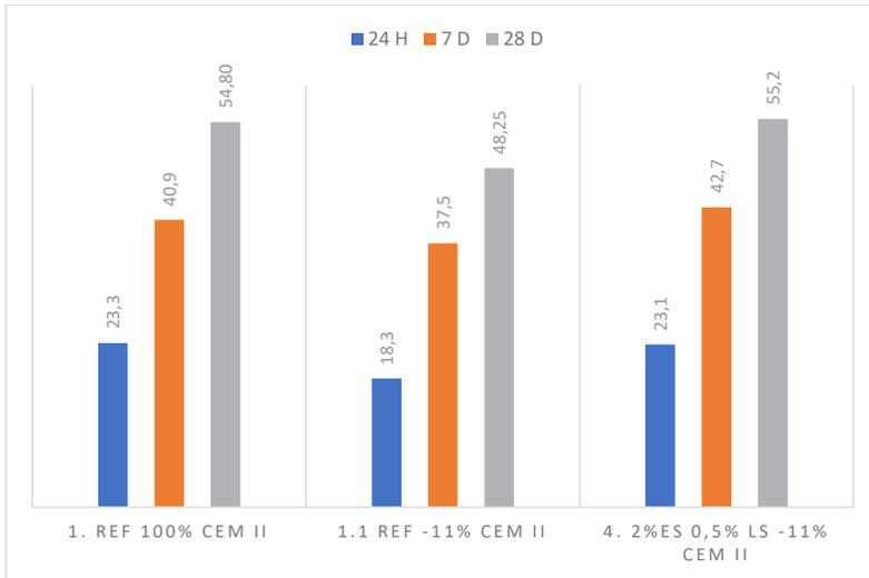
Figure 4 positive effects of Ls accelerator
