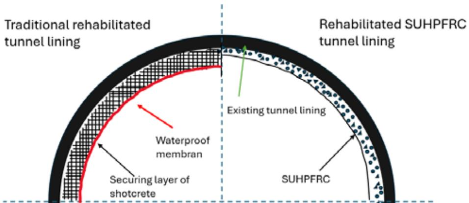
Figure 2: Functional requirements of a dry surface possibly achieved by traditional methods and SUHPFRC.
