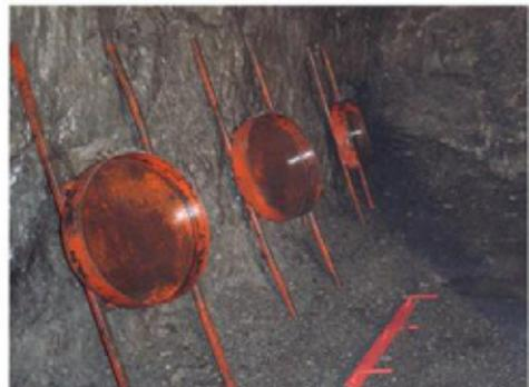
Picture 1 and 2: Circular Energy-absorption test panel forms [1].
