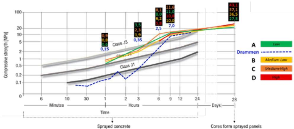
Figure 5 – Comparison of early age strength development between the four final mixes tested and the Drammen mix
