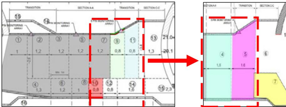
Figure 6 – SCL construction sequence based on poor (LHS) and stable (RHS) ground conditions
