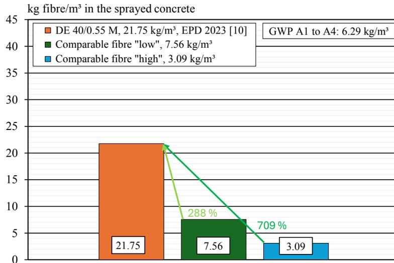
Figure 6 – Maximum dosage for reaching the same GWP A1 to A4 of 6.29 kg/m<sup>3</sup> sprayed concrete
