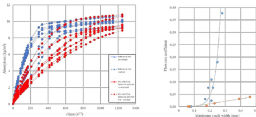
Figure 8 - Effect of cracking on capillary suction (left) and steady-state flow in cracks (right) for reference mix and mix with polymer [14].
