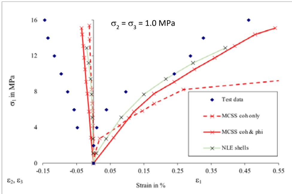
Figure 3 Triaxial test on sprayed concrete with predictions from various numerical models & experimental data (after [3]). 1 = the direction of loading & 2,3 = the lateral directions; positive strains are inwards to the centre of the sample.
