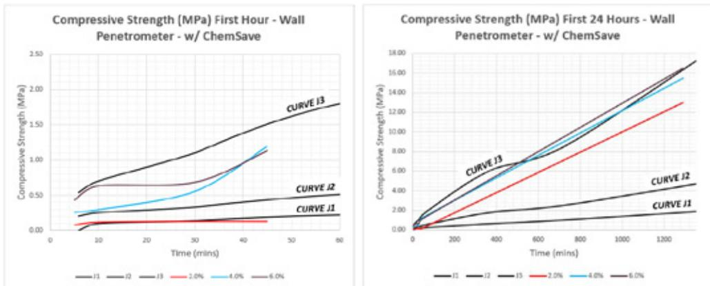
*Figures 3 & 4 – Compressive Strength of Sika MS-WIUG product using Sigunit L-500 Accelerator at varying dosages using ChemSave system*
