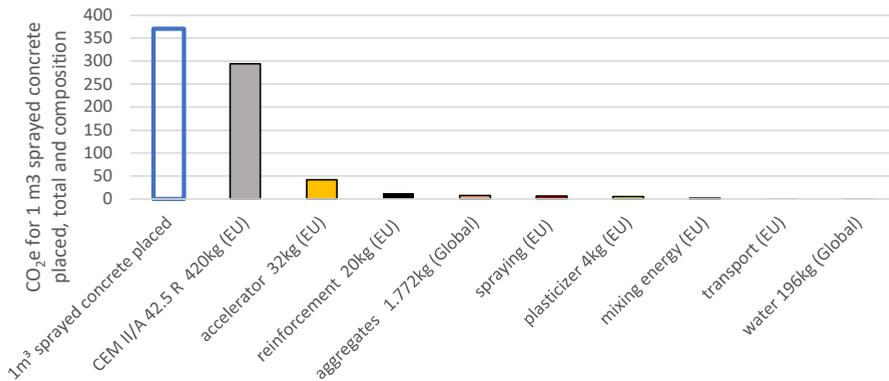
Figure 1: CO<sub>2</sub>e for 1m<sup>3</sup> applied sprayed concrete – relevance of CO<sub>2</sub>e contributors [5]
