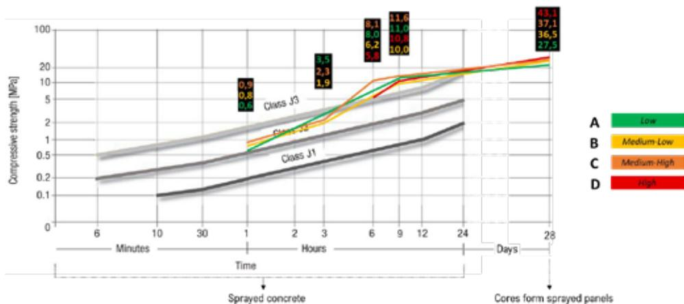
Figure 4 – Early age strength development measured after spraying
