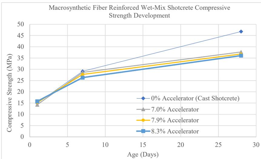
Fig. 3 Compressive Strength Development for Macrosynthetic Fiber Reinforced Wet-Mix Shotcrete
