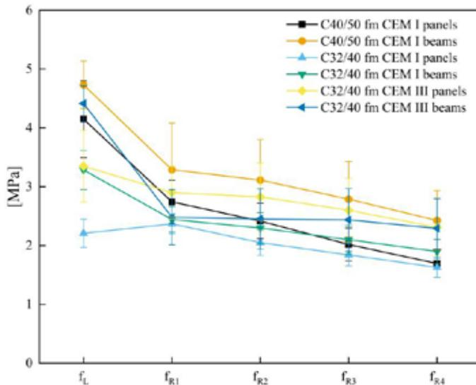
Figure 4 - C40/50 and C32/40 CEM I & CEM III B Dramix® 4D 65/35BG fibre panel and beam mean flexural tensile strengths
