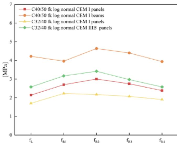
Figure 5 - C40/50 and C32/40 CEM I & CEM IIIB Dramix® 3D 80/30BGP fibre panel and beam characteristic flexural tensile strengths
