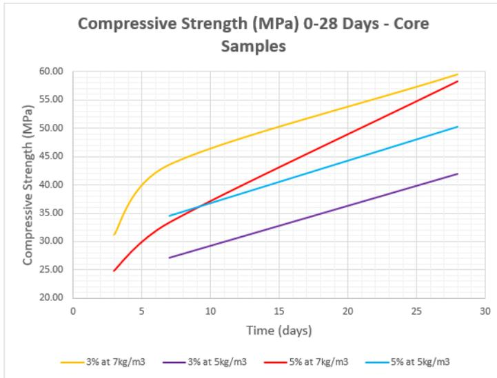
Figure 6 – Core Sample Test Results for 28-Day Compressive Strength Development of a Fibrecrete Material
