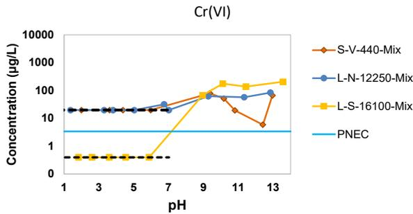
Figure 3 - Leaching as a function of pH for Cr(VI). Quantification limits are indicated as QL (Quantification Limit) with horizontal dashed lines from pH < 7.0. The second last basic data point on each measurement series is the material pH. PNEC is the predicted no-effect concentration.
