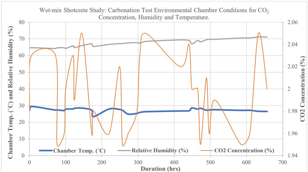
Fig. 1 Environmental Conditions for Test: (Temperature, Relative Humidity) and CO<sub>2</sub> Concentration Values Recorded.
