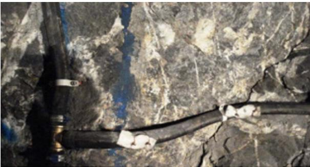
*Figure 4 - Detailed image of the piping system: the vertical water supply pipe is on the far left, with the horizontal, perforated pipe for water permeation visible on the right.*
