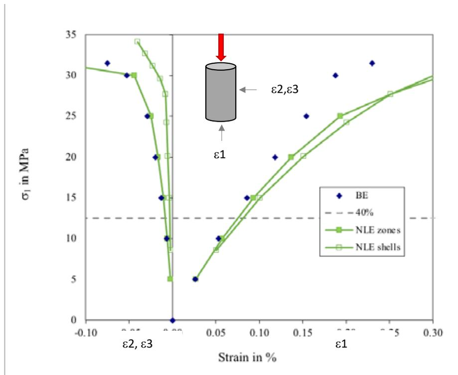
Figure 1 Uniaxial compression test on sprayed concrete from the Brite Euram (BE) project with predictions using a nonlinear elastic model (NLE) with either zones or shell elements (after [3]). 1 = the direction of loading & 2,3 = the lateral directions; positive strains are inwards to the centre of the sample.
