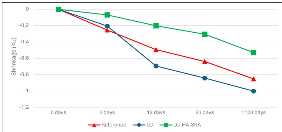
Figure 4 – Development of shrinkage over time.
