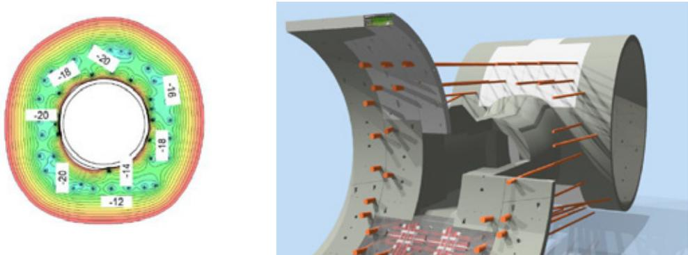
Figure 2 – Freeze zone with a minimum temperature of  $-10^{\circ}\text{C}$  (LHS), AGF at CP (RHS)
