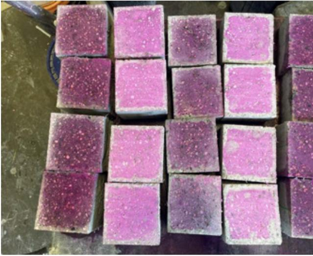
Fig. 2 Carbonation penetration depth being measured for wet-mix shotcrete
