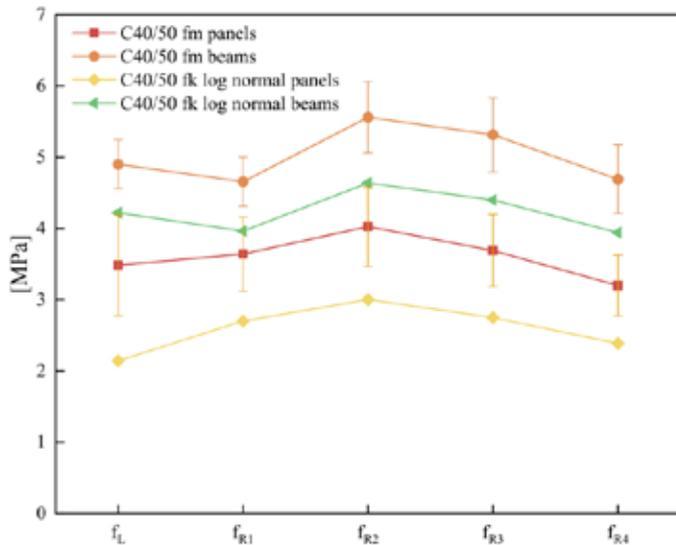
Figure 3 - C40/50 CEM I Dramix® 3D 80/30BGP fibre notched panel and beam mean and characteristic flexural tensile strengths
