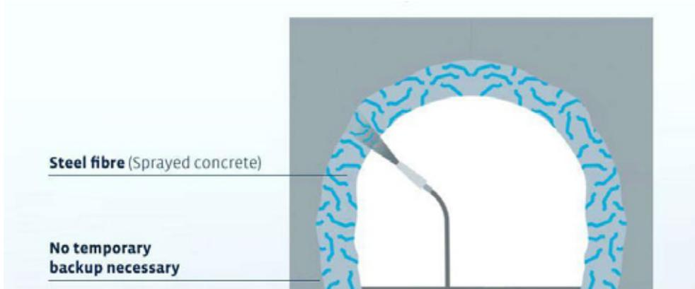
Figure 1 - Solution with steel fibre reinforced sprayed concrete [3]
