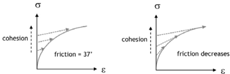
Figure 2 Schematics showing options for setting Mohr-Coulomb parameters: a) cohesion increase while friction is constant and b) cohesion increase while friction decreases
