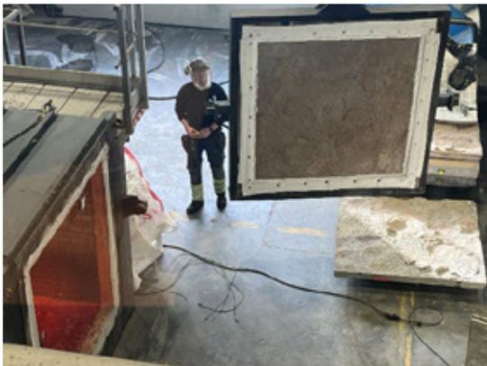
Figure 2 (top) HC fire curve (red dotted line) and measured own temperatures [20] during the eight sprayed concrete element tests. (bottom) Fire test own and test element.
