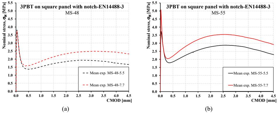
Figure 3. Comparison of mean experimental curves in terms of fibre contents for a given fibre type: MS-48 panels (a) and MS-55 panels (b).
