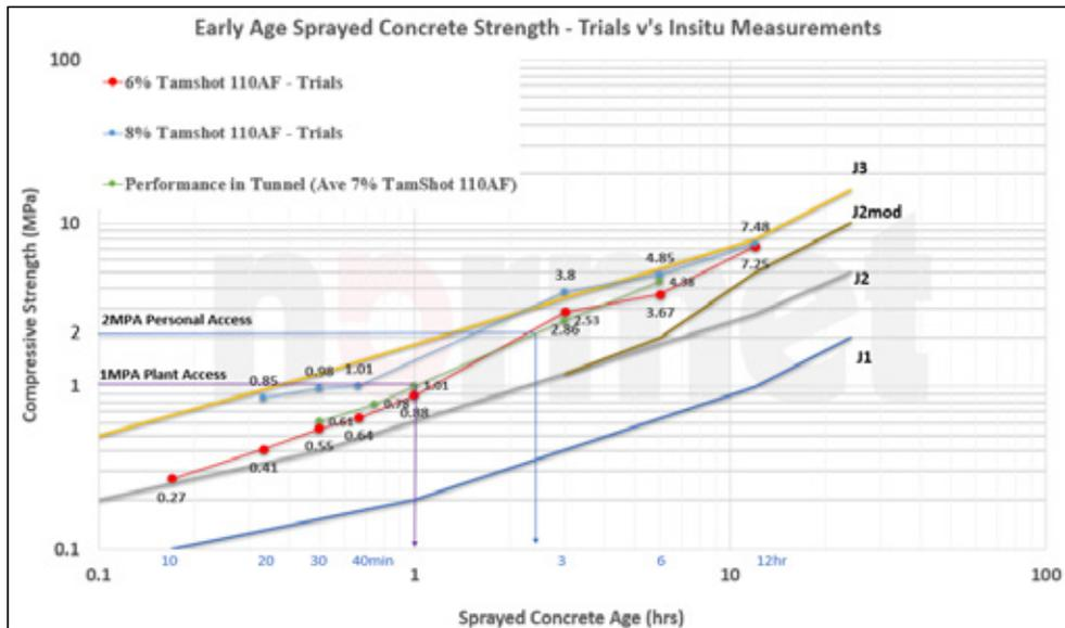
Figure 3 – EAS results: Insitu testing vs. surface trials
