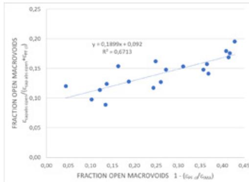
Figure 6 - Fraction of open macro voids measured by two methods, see eq. (1) and (2)
