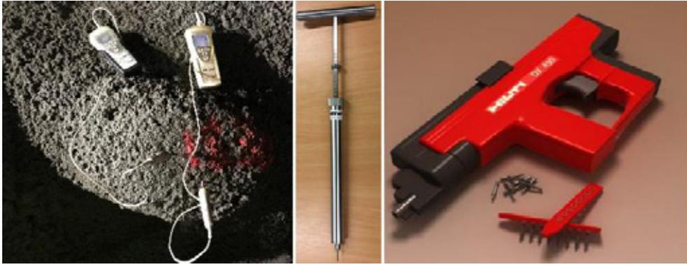
Figure 1 - Left: Temperature measurements on sprayed concrete. Middle: Example of needle penetrometer. Right: Hilti gun for the Hilti gun method.
