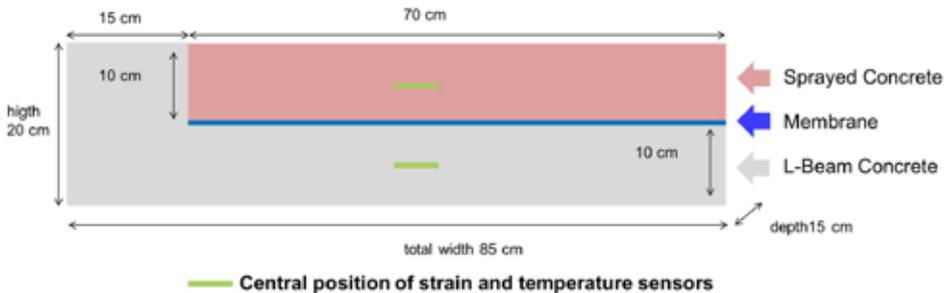
Figure 5 - Schematic drawing of the cast L-beam as base, with sprayed membrane and sprayed concrete.
