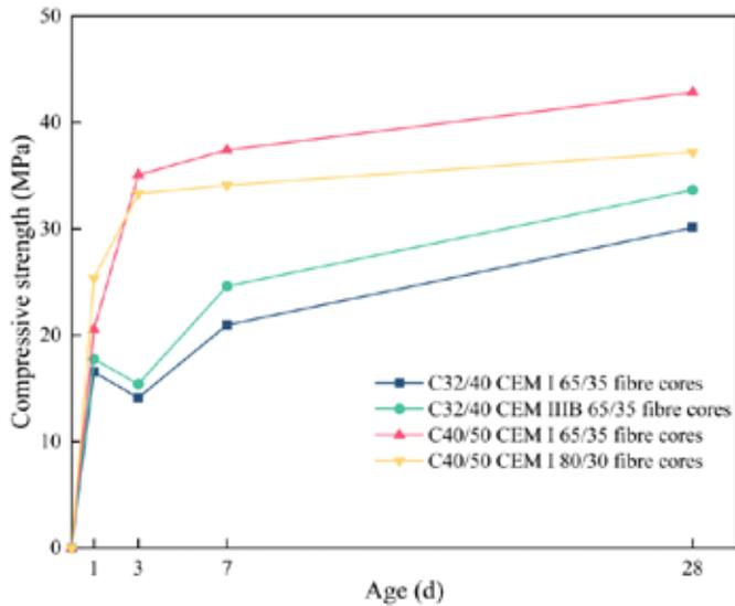
Figure 1 C40/50 and C32/40 CEM I & CEM III B core compressive strength development
