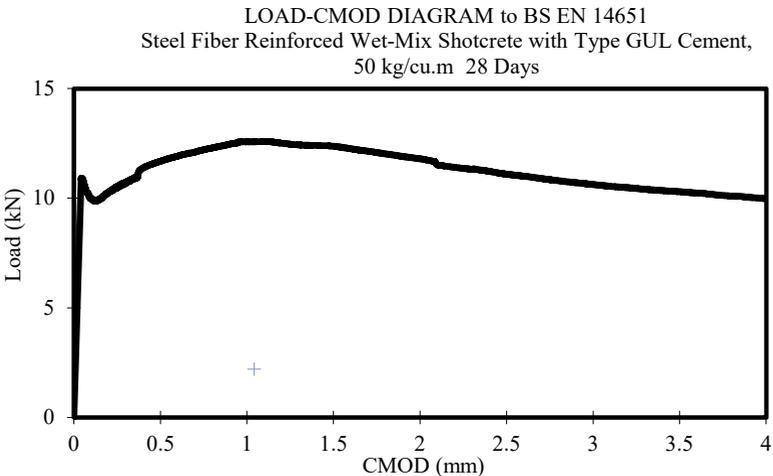
Fig. 8 Load vs. CMOD for Steel Fiber Reinforced Wet-Mix Shotcrete Notched Beam tested to BS EN14651
