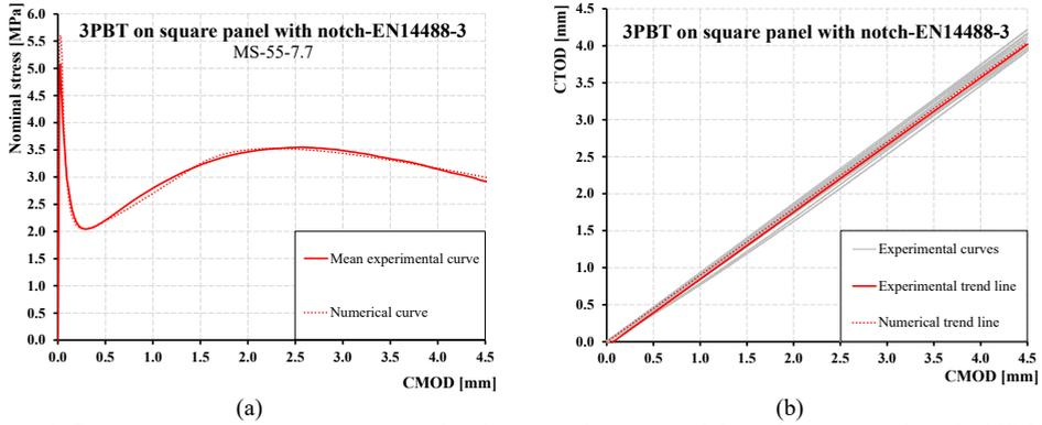
Figure 6. Comparison: mean curves experimental and numerical as retrieved through inverse analysis for MS-55-7.7 series (a) and numerical vs. experimental trend lines CTOD vs. CMOD (b).
