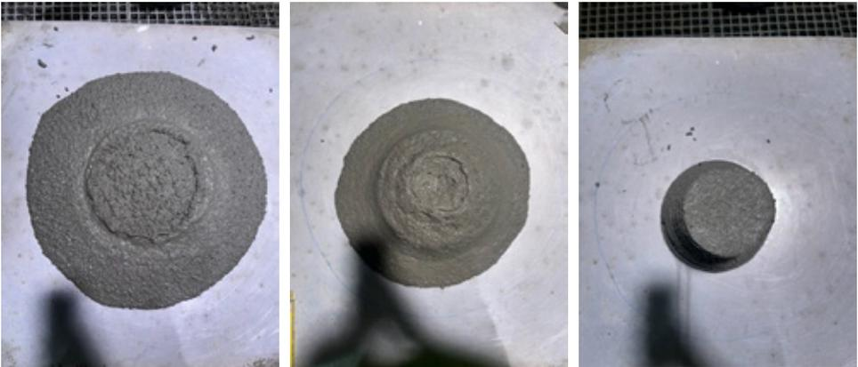
Figure 2: Concrete mix 4.1 initially after mixing, after 1 hour and after 2 hours.
