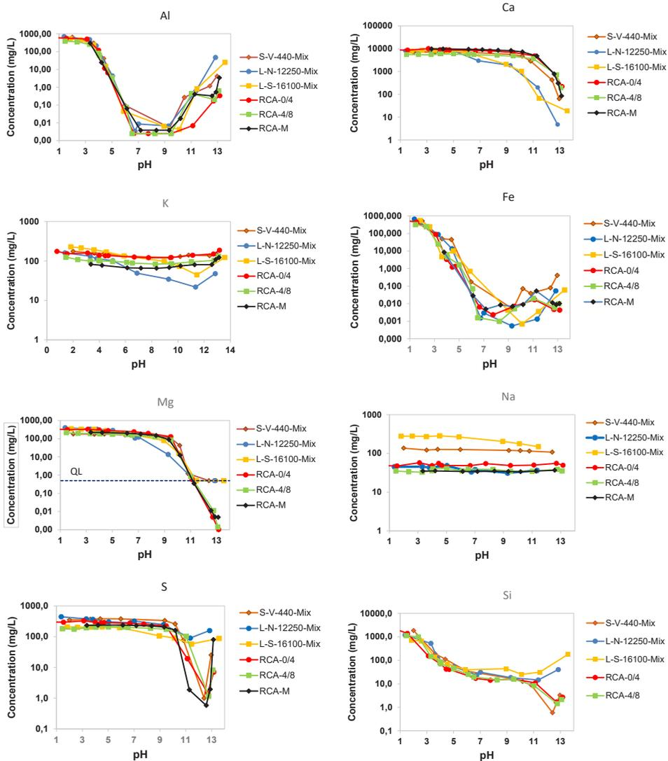
Figure 1 - Leaching as a function of pH. The quantification limit for Mg in this study is indicated as QL (Quantification Limit) with a horizontal dashed line. The second last basic data point on each measurement series is the material pH. For Na, the material pH is the last data point. RCA 0/4 (crushed concrete), RCA 4/8 (crushed concrete) and RCA-M (crushed mortar prism) are leaching from crushed concrete and mortar from previous studies [6], [7].
