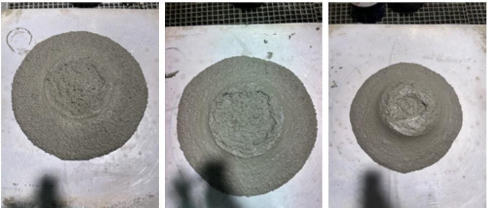
Figure 3: Concrete mix 5.1 initially after mixing, after 1 hour and after 2 hours.
