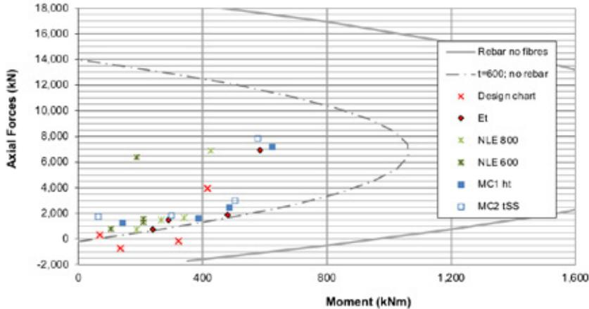
Figure 5 Lining loads vs capacity at a large diameter SCL tunnel junction after [6]
