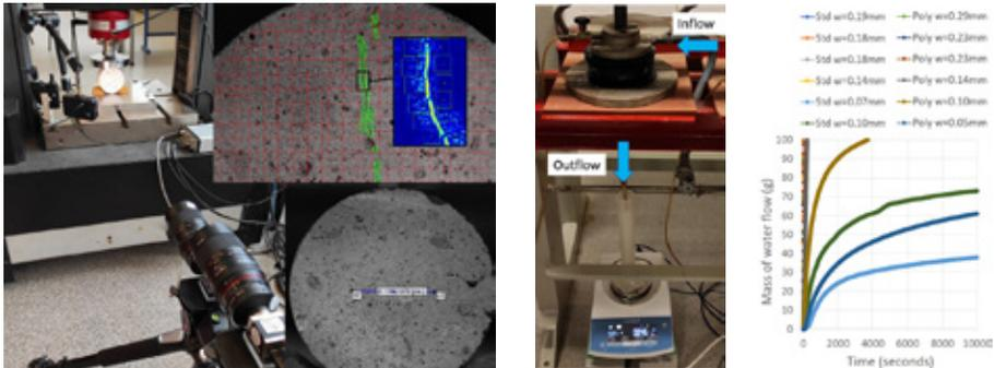
Figure 4 - crack flow experiment with DIC-controlled crack-width (w) in Brazilian test and crack-width analysis (left), steady-state water crack-flow experiment (centre) and flow plot (right)
