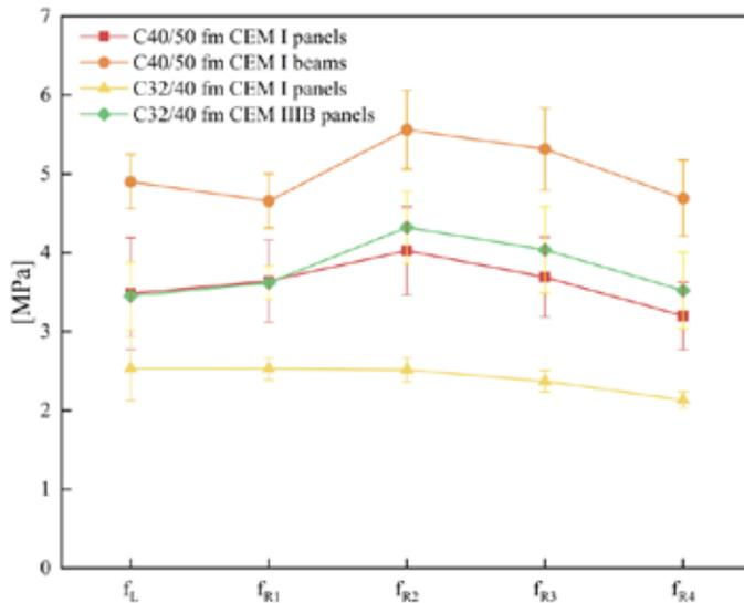
Figure 6 - C40/50 and C32/40 CEM I & CEM III B Dramix® 3D 80/30BGP fibre panel and beam mean flexural tensile strengths
