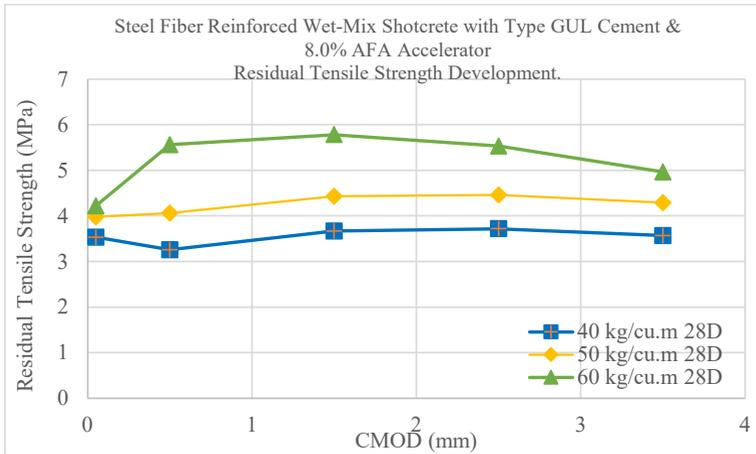
Fig. 9 Residual tensile strength test for steel fiber reinforced wet-mix shotcrete
