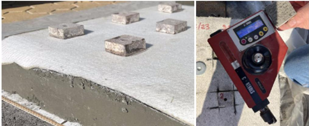
Figure 7: notches glued to the external (extrados) surface of the waterproofing membrane on the shotcrete sample-box (left), digital dynamometer used during the adhesion strength (pull-off) test (right).
