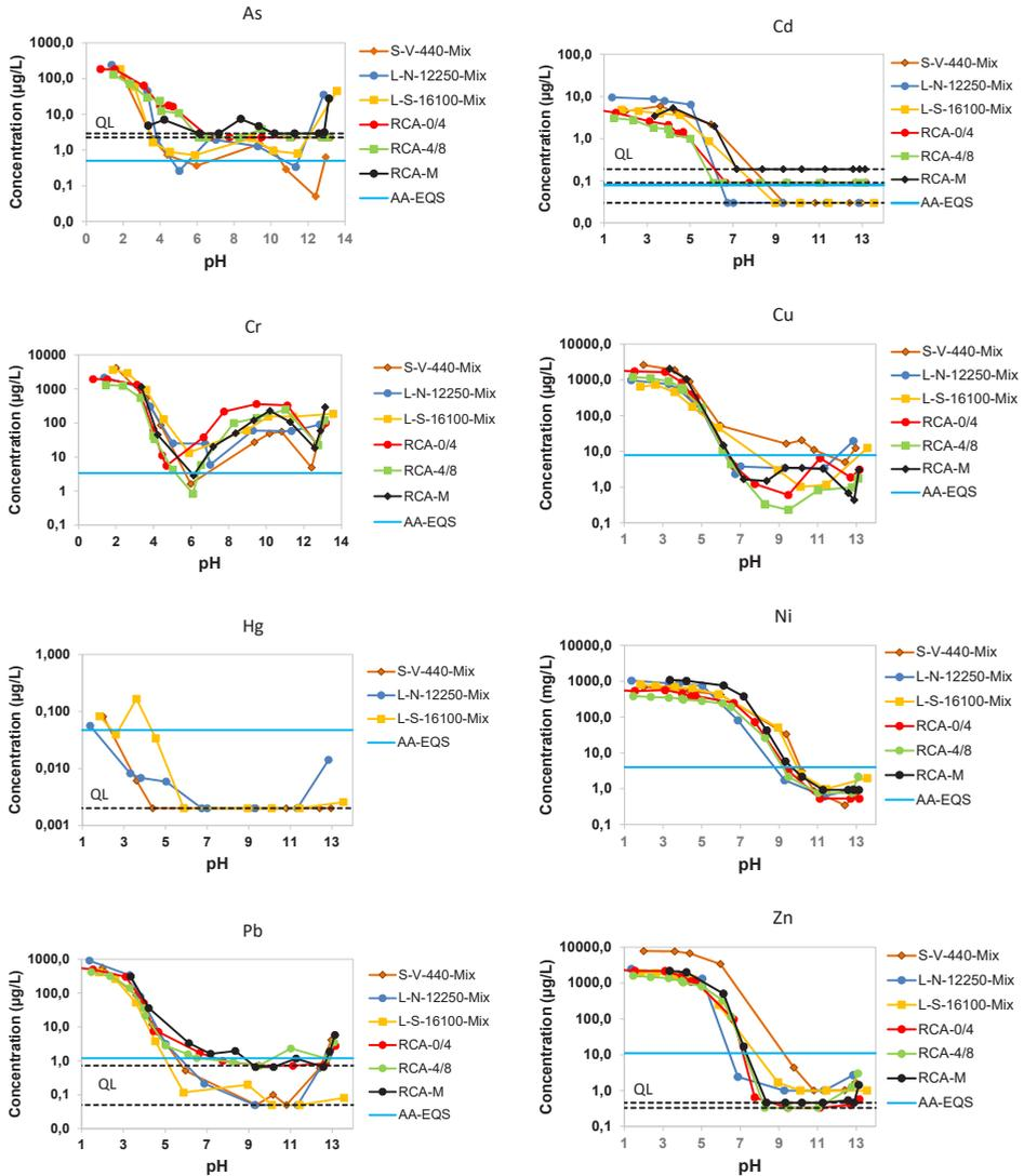
Figure 2 - Leaching as a function of pH for As, Cd, Cu, Cr, Hg, Ni, Pb and Zn. Quantification limits are indicated as *QL* (Quantification Limit) with horizontal dashed lines. The second last basic data point on each measurement series is the material pH. AA-EQS is the Annual Average Environmental Quality Standard. RCA 0/4 (crushed concrete), RCA 4/8 (crushed concrete) and RCA-M (crushed mortar prism) are leaching from crushed concrete and mortar from previous studies [6], [7].
