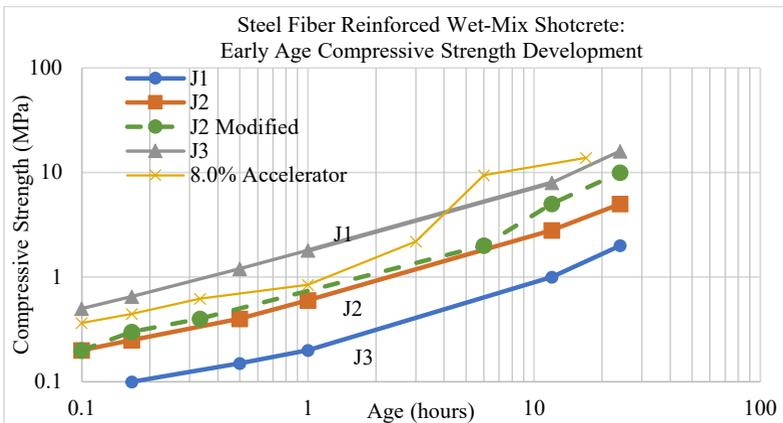
Fig. 2 Early Age Compressive Strength Development for Steel Fiber Reinforced Wet-Mix Shotcrete
