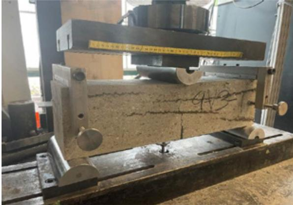
Fig. 5 Fiber Reinforced Wet-Mix Shotcrete Notched Beam tested to BS EN14651
