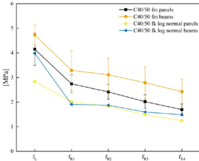
Figure 2 - C40/50 CEM I Dramix® 4D 65/35BG fibre notched panel and beam mean and characteristic flexural tensile strengths
