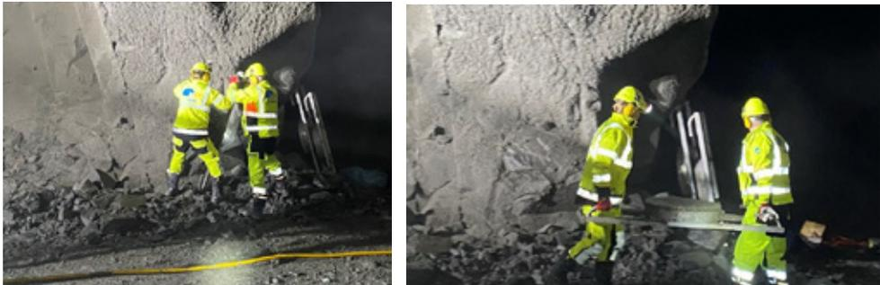
Picture 5 and 6: Loose the EATP-form from the wall after spraying, and then carry it manually and carefully to the location where samples are treated.
