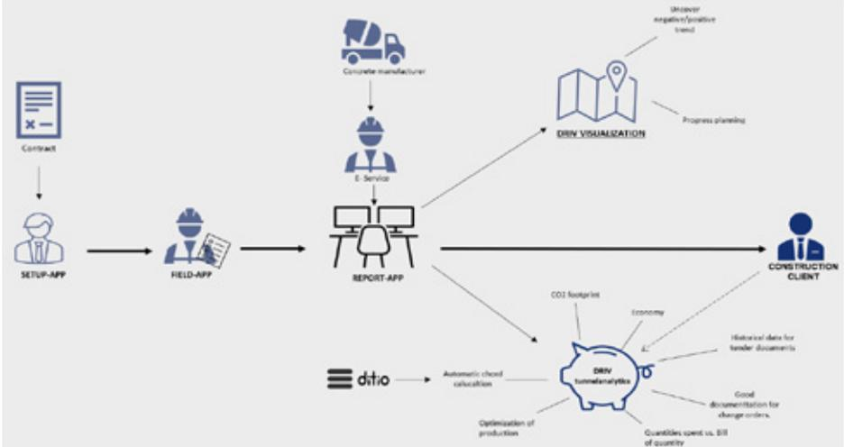
**Figure 1. Dataflow in DRIV from SETUP to construction client**
