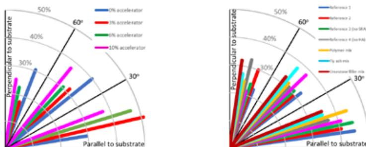
Figure 7 - Orientation of length axis of macro voids Flekkefjord (left) and Svorkmo (right)
