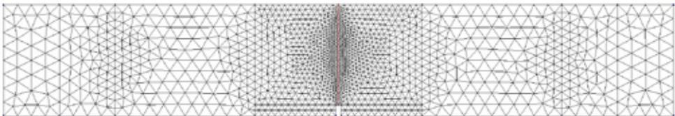
Figure 5. Mesh adopted with evidenced interface elements used for the discrete mid-span crack.
