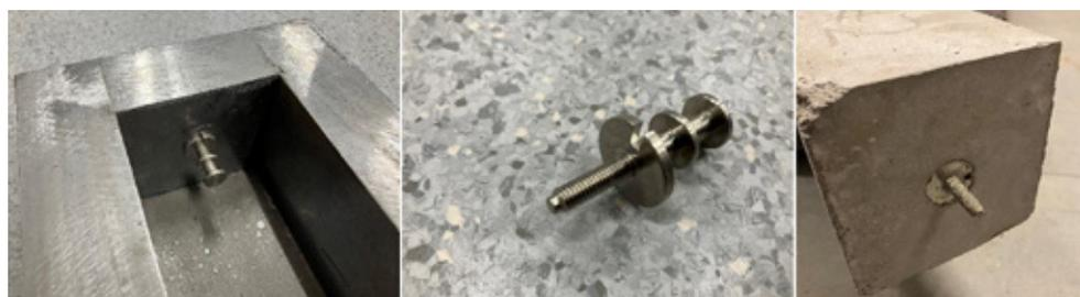
Figure 3 – Left: mould. Middle; closeup of steel peg. Right: close-up of sprayed specimen.
