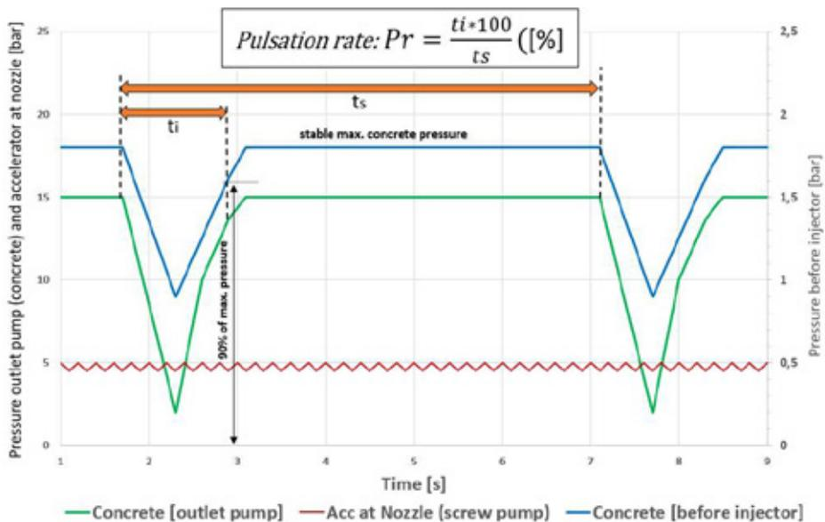
Figure [3]: Typical pressure development during the operation of a sprayed concrete pump (graphic-based on [8])
