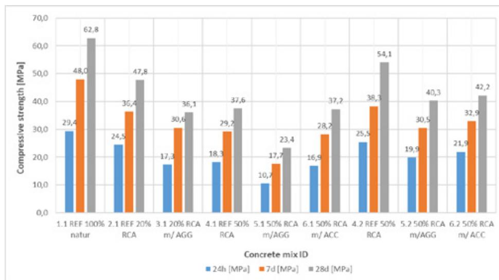
Figure 4: Compressive strength after 24 hours, 7 days and 28 days for all concrete mixes.
