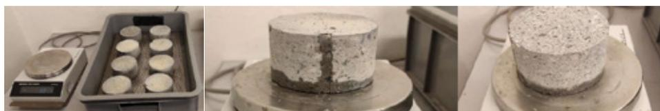
Figure 2 - One-sided capillary suction experiment (left) on slices of wet sprayed concrete from drilled cores, with (centre) and without (right) crack.
