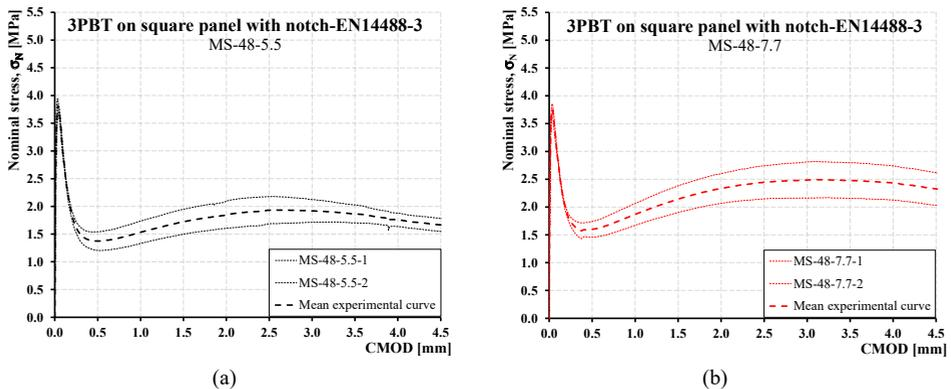
Figure 2. Experimental results of MS-48 panels with evidenced mean experimental curves: 5.5 kg/m<sup>3</sup> ( $V_f=0.60\%$ ) (a) and 7.7 kg/m<sup>3</sup> ( $V_f=0.85\%$ ) (b).
