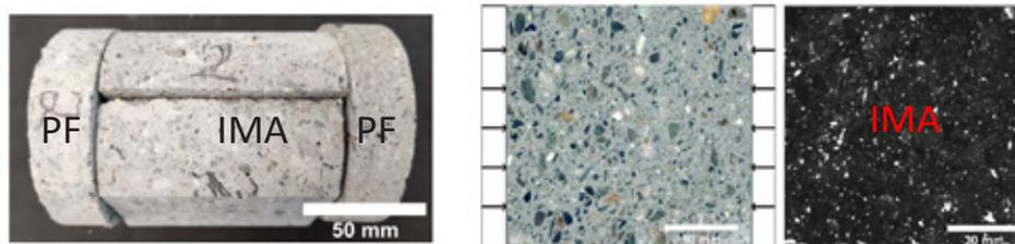
Figure 1 - Specimens for capillary suction/PF and for IMA (polished, coloured black-white)
