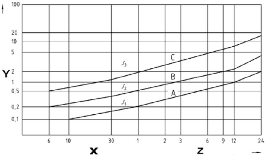
Figure 5: compressive strength development curves in the first 24 hours, according to EN 14487-1.
