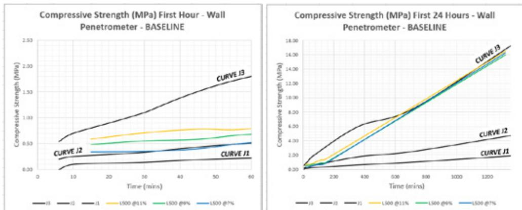
*Figures 1 & 2 – Field Data for Compressive Strength of MS-WIUG product using Sigunit L-500 Accelerator*
