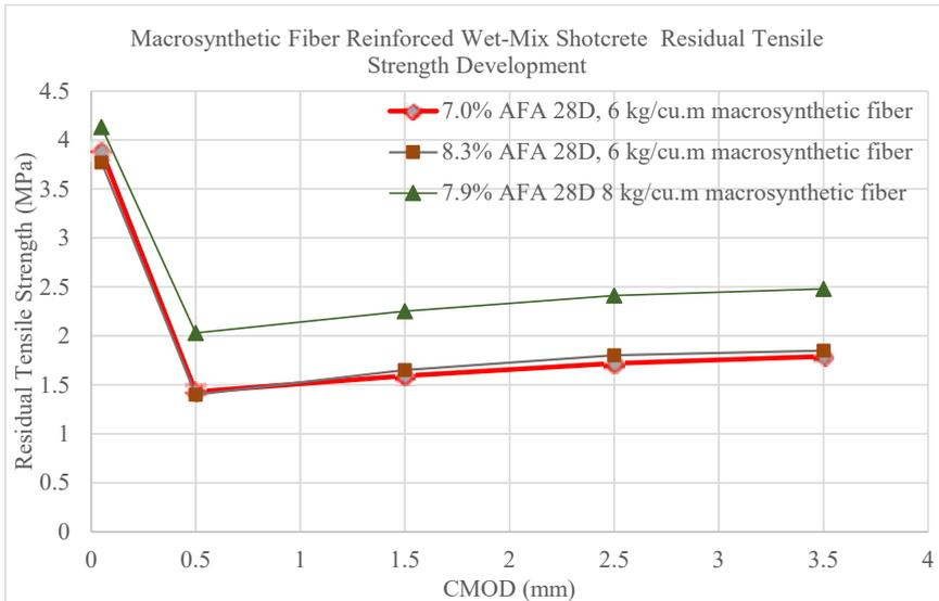
Fig. 7 Residual Tensile Strength for Macrosynthetic Fiber Reinforced Wet-Mix Shotcrete tested to BS EN14651
