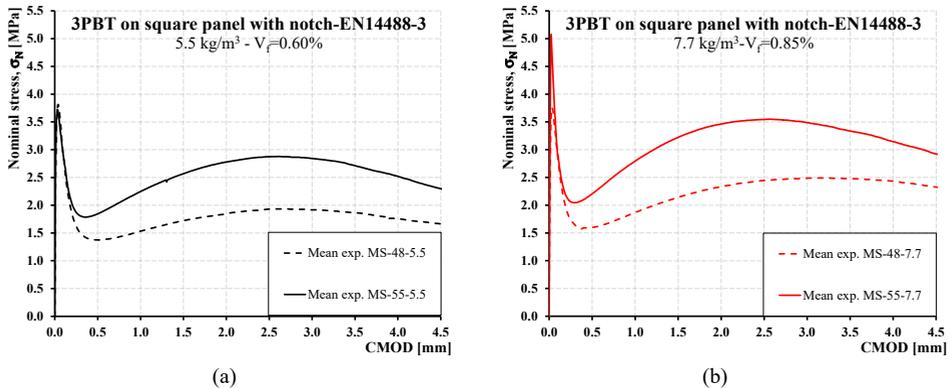
Figure 4. Comparison of mean experimental curves in terms of fibre aspect ratio for a given fibre content: 5.5 kg/m<sup>3</sup> ( $V_f=0.60\%$ ) (a) and 7.7 kg/m<sup>3</sup> ( $V_f=0.85\%$ ) (b).
