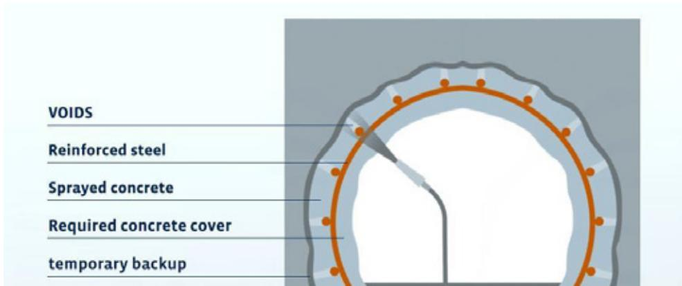
Figure 2 - Solution with conventional reinforced sprayed concrete [3]
