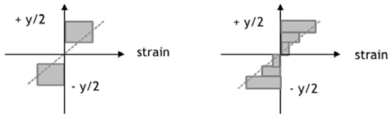
Figure 4 Schematic of the approximation of strain in pure bending through the section of a beam a) using 3 constant strain zones and b) 6 constant strain zones vs simple beam theory (dashed line)
