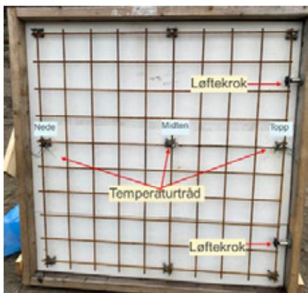
Figure 4 Element formwork with PE-foam at the rear side, mesh reinforcement in center, thermo-couple locations and lifting anchors. Final locations during later fire test: topp=top, midten=center, nede=bottom.
