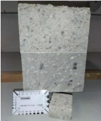
Figure 6 - Cross-section of the L-beam, showing the spray-applied membrane lining in the center and the sprayed concrete on top.
