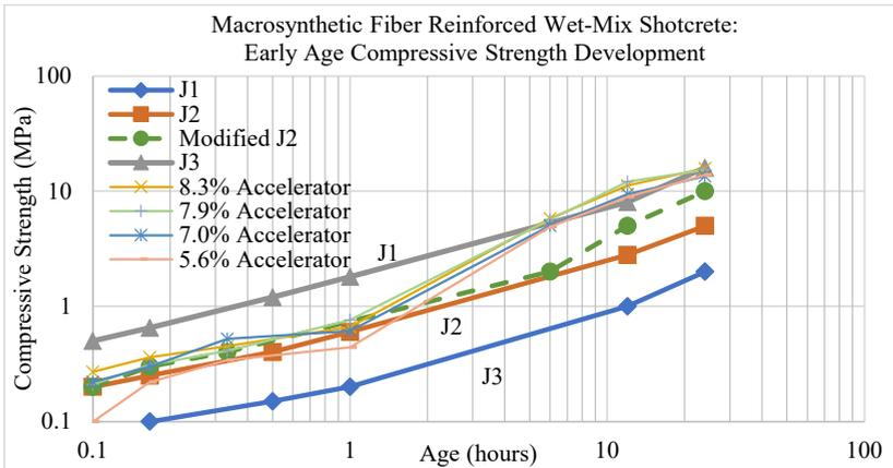
Fig. 1 Early Age Compressive Strength Development for Macrosynthetic Fiber Reinforced Wet-Mix Shotcrete
