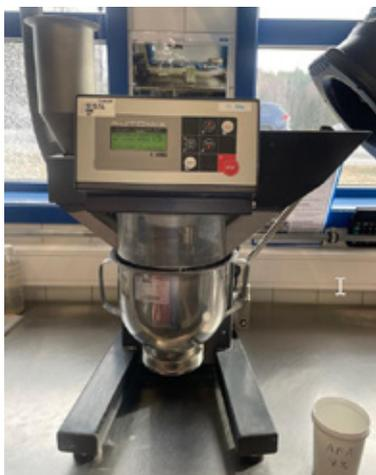
Figure 1 The Controls auto mixer, used for the mix of plastic mortar.
