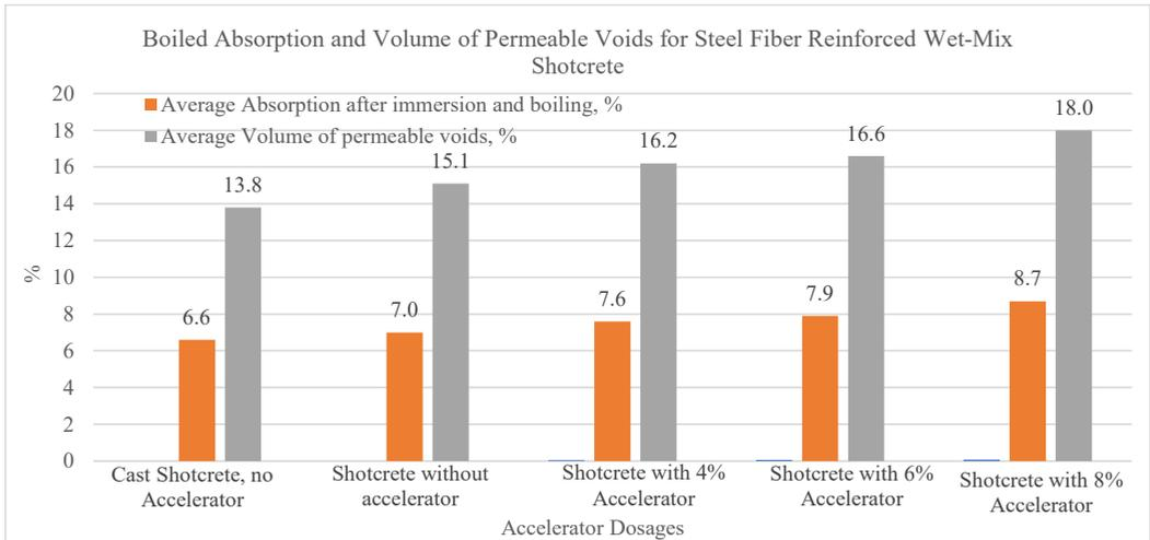
Fig. 3 Boiled Absorption and Volume of Permeable Voids for Steel Fiber Reinforced Wet-Mix Shotcrete
