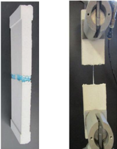
*Figure 7, left - Test piece after stripping; the fiber is embedded in the center of the test piece and stabilized by polyethylene foam.*
