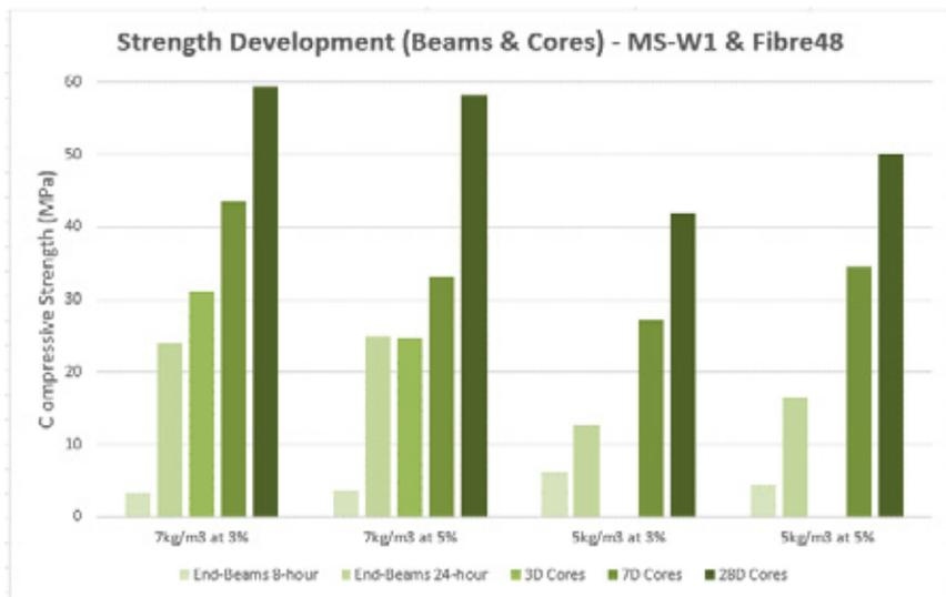
Figure 7 – Strength Development Results for End-beam & Core Test Samples
