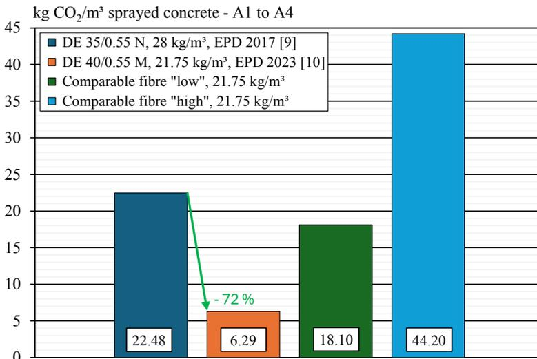
Figure 5 – Comparison of the GWP – A1 to A4 - in kg CO<sub>2</sub>/m<sup>3</sup> sprayed concrete of different fibres
