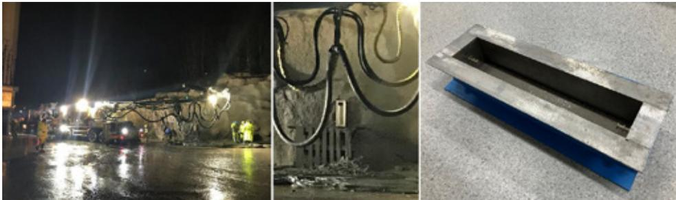
Figure 2 – Left: Full-scale test of sprayed concrete Middle: spraying of specimens for shrinkage measurements. Right: Mould for shrinkage measurements.
