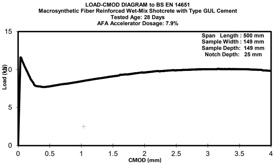
Fig. 6 Load vs. CMOD for Fiber Reinforced Wet-Mix Shotcrete Notched Beam tested to BS EN14651
