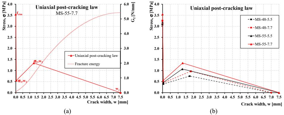
Figure 7. Typical uniaxial post-cracking law with evidenced main parameter and development of  $G_f$  (a) and post-cracking uniaxial constitutive laws of all series investigated (b).
