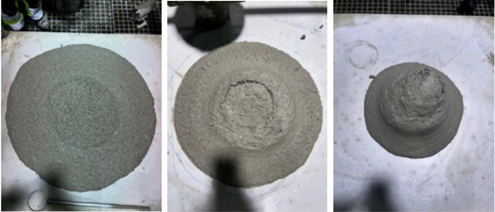
Figure 1: Concrete mix 1.1 initially after mixing, after 1 hour and after 2 hours.
