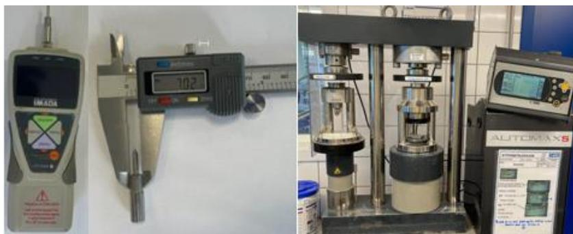
Figure 2 showing Imada penetrometer, the needle for Imada for compression <0.5MPa and the compressive strength machine. for > 0.5 MPa.
