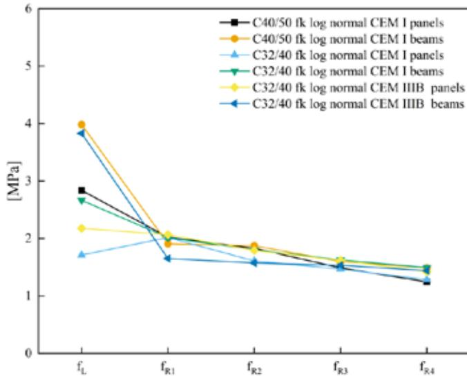
Figure 5 - C40/50 and C32/40 CEM I & CEM III B Dramix® 4D 65/35BG fibre panel and beam characteristic flexural tensile strengths
