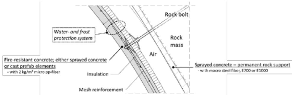
Figure 1 Typical build-up of a Norwegian tunnel (based on [2]): First, sprayed concrete permanent rock support (with separate bolting according to the rock mass class) produced according to [3]. Then, an inner lining of water- and frost protection including insulation and mesh-reinforced fire-resistant concrete.
