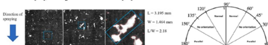
Figure 3 - Measurement of Length/Width ratio and quantifying orientation of macro voids
