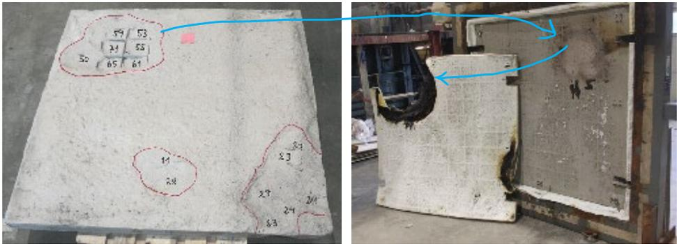
Figure 8 After completed fire test; 50  $\mu$ m - 1,5 kg, sprayed concrete element: Exposed side of element (left) and backside with insulation (right).
