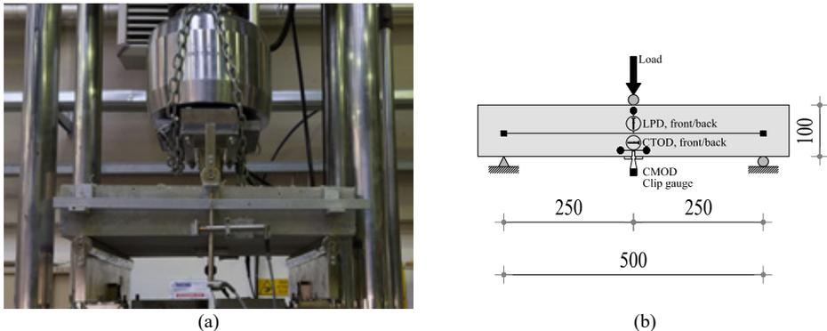
Figure 1. Test set-up (a) and instrumentation details (b) of square panels with notch tested according to EN 14488-3 [8] (dimensions in mm).
