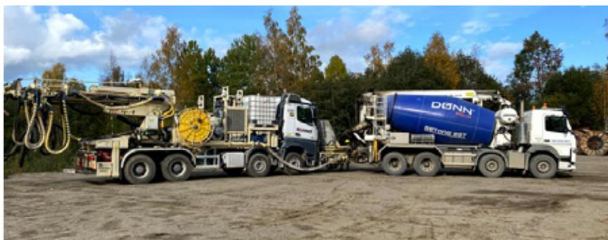
Figure 3 Concrete delivering and equipment for spraying.
